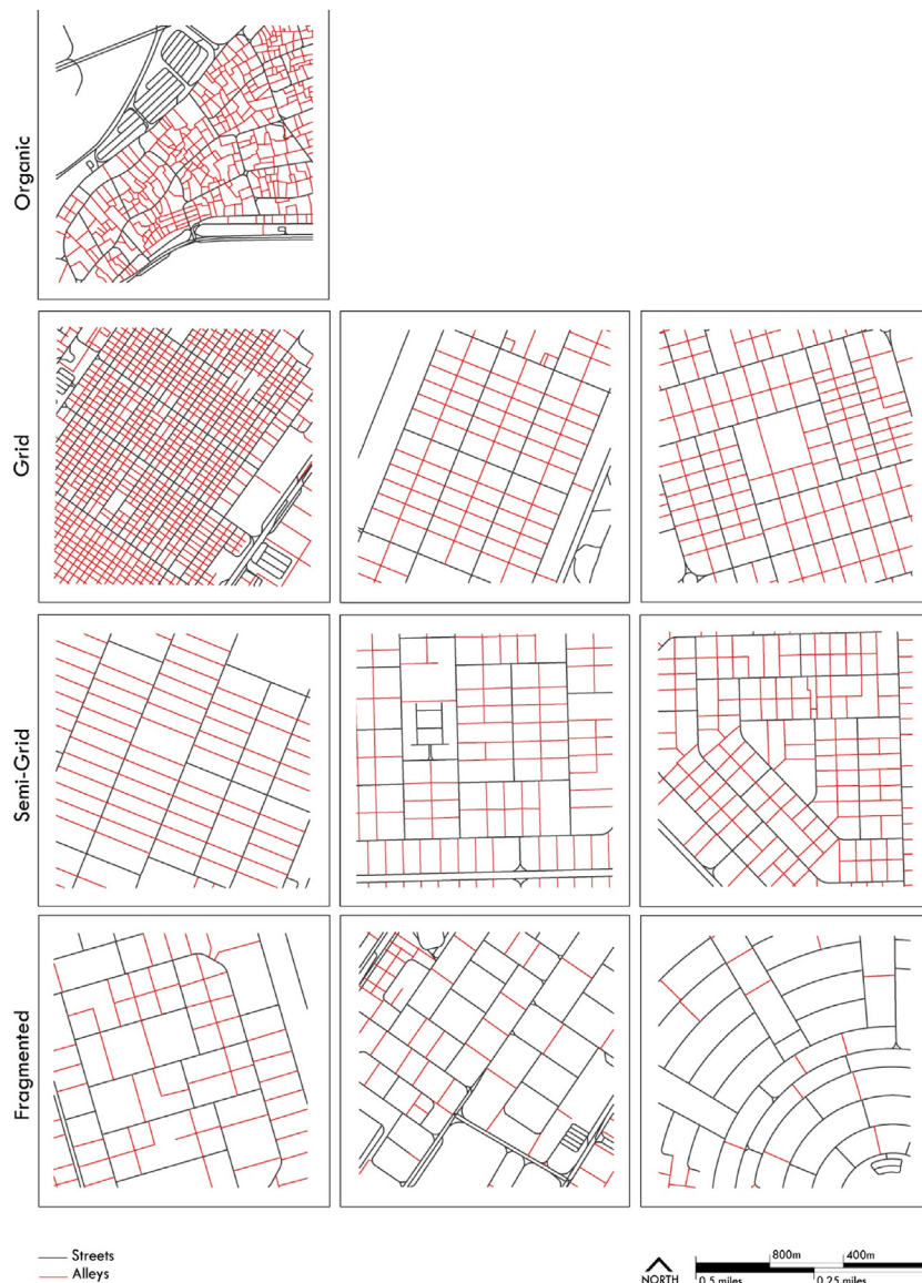
Fig. 4. Alleys typologies (from top row to bottom row): Organic, Grids, Semi-grids, and Fragmented. Organic alleys are usually found in old settlements that evolved without any formal planning interventions. Grid alleys resemble the grid network of streets with a high number of four-way intersections. If a layout closely resembles a grid but has dead ends and multiple T-intersections forming some disconnections in the network, it is identified as a semi-grid network. Fragmented layouts have sporadic presence of alley segments with minimal continuity.
